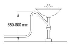
The drain hose can be connected directly into the pipe (e.g. beneath a washtub or sink), above the water trap. The drain hose must be arranged so that some part of it's length is routed up to a level corresponding to the top edge of the tub and fixed in place there.
